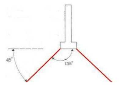
The "angle of repose", red lines, show distinctly the critical area in which you **must not** dig or tunnel. Disturbing the soil anywhere within those boundaries could lead to serious, and difficult to repair, consequences.
